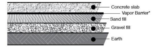
\*Fortifiber "Moistop" vapor barrier placed over tamped fill directly beneath concrete slab (800/773-4777) On 1 layer of 10 mil black polyurethane or black vinyl membrane or 2 layers of 6mil
